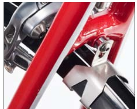
Figure 15. Fender bridge clip held by interior screw
